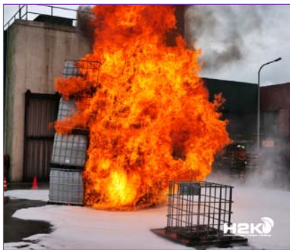
Image 16: composite pallets weaken at location of the leak
