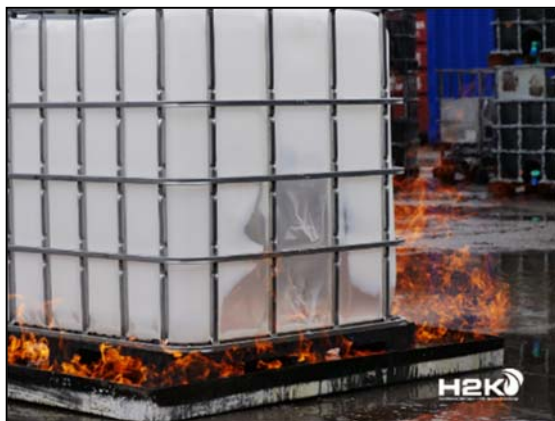
Image 9: Translucent spot CIBC weakens and fails
