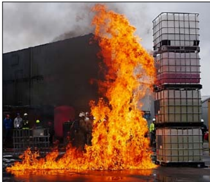
Image 14: stack four CIBCs with integrated composite pallets. Burning liquid from top CIBC at early stage of fire
