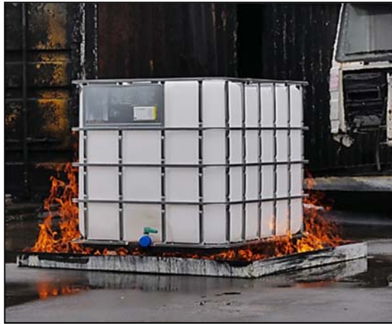
Image 7: after liquid was ignited in tray
