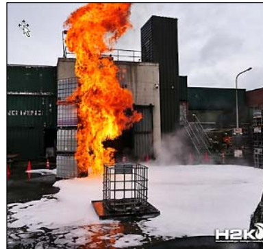
Image 15: fire on surface below stack is kept under control with foam
